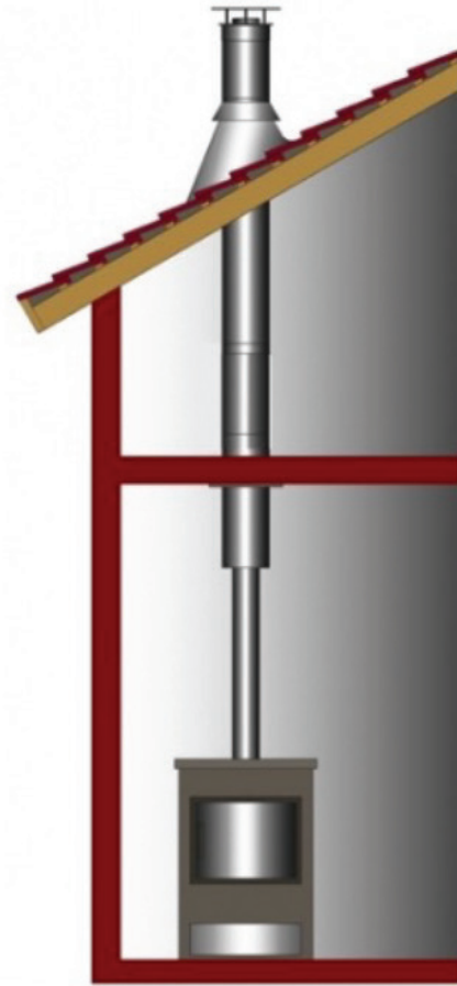
Figure 5: Steel pipe chimney. Note the lower part is not insulated.
